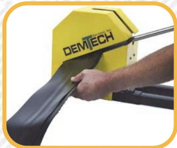
The Bone-Cutter provides easy loading of both fusion or extrusion welds.
