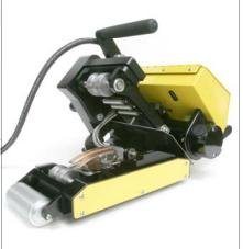
The wedge assembly can be **removed in 30 seconds** by simply unplugging the external heater and thermocouple plug-in wire connector, removing two shoulder bolts, and opening up the frames as shown above. Just lift the wedge assembly and pull it out!
