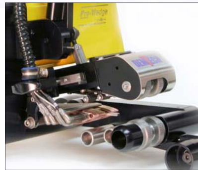
In disengaged position, wedge and nip rollers offer plenty of clearance, reducing burn-outs at beginning of seam when welding thin materials.
